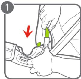
1 To attach canopy, insert the canopy bow into the canopy mounting brackets on both sides of the seat until it clicks into place. Pull canopy over back of infant restraint.
