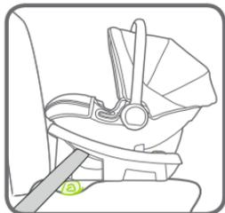
9 To remove base from vehicle seat, push in on the UAS connectors red buttons and remove.
