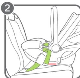
2 Check the red line level on the side of the shell to make sure it is level to the ground.
