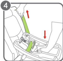
4 While pressing the base down into the seat, pull on the vehicle belt to tighten.
